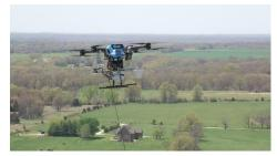
Earlier this month, AT&T announced that their drone operations team has achieved an industry first in transmitting its 5G network via a drone. The test was performed in April in rural Missouri with AT&T's so-called "Flying COW," or Cell on Wings. These Flying COWs have been operating since 2017 to provide LTE connectivity
