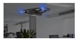
Tando uses multiple sensors and proprietary algorithms to map and navigate in any indoor space. The drone can autonomously navigate above or around any items in its path, which allows it to secure and monitor large areas. When it's not in flight, the drone docks on a charging and monitoring station mounted on the ceiling and
