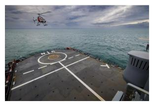
The test campaign used an optionally piloted vehicle based on a modified Guimbal Cabri G2 equipped with the autonomous take-off and landing (ATOL) system developed for the VSR700. The VSR700 is being developed by the French Armament General Directorate for France's Navy as part of its Système de drone aérien de la Marine program.
