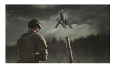
The new loitering munition weighs 50lb, is man-portable and can be set up for deployment from a launch tube in less than 10min. It also can be configured for launch from a vehicle or slow-moving aircraft.
