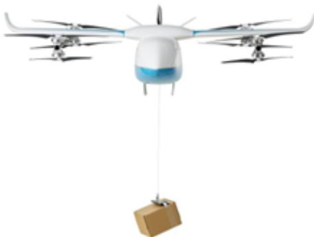
The RDSX Pelican uses a hybrid VTOL design that can handle up to 5 kg payloads on up to 40 km routes.
