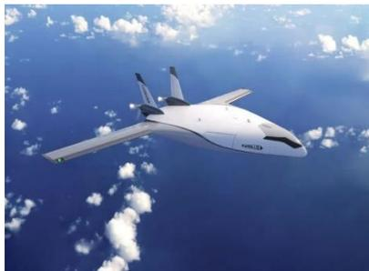
Hydrogen-electric propulsion company ZeroAvia has teamed with Natilus, which has designed an autonomous blended wing body cargo plane that might offer some advantages in making a commercially viable aircraft. The spacious interior of the Kona has more room to store hydrogen than conventional designs and that might tip the balance in getting the range necessary to make a useable aircraft.
