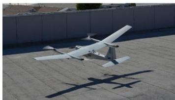
AeroVironment has expanded the capabilities of its successful Puma SUAS with the introduction of a VTOL kit. This enhancement to the 3 AE (all environment) model allows for a shift from fixed-wing to VTOL in minutes, expanding operational capabilities in urban and/or GPS-denied navigation in contested spaces.
