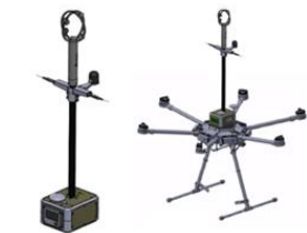
Figure 2. TriSonica system integrated with Bluebird's Meteorological Characterization Payload (MCP) attached to a VLOS Weather Air (left)
