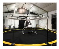
release in 2023. It has 18 propellers, nine batteries, and it has a flight time rated at 30 minutes. Volocopter has redundancies and even emergency parachutes for its two passengers, but the microprocessors that monitor the environment for turbulences and winds were implemented for a safe and smooth flight. Besides the ongoing test flights in Dubai, Volocopter received a permit to fly in Germany, where it flies regularly.
