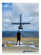
Martin UAV provided surveillance and reconnaissance for USSOUTHCOM during the mission, deploying EO/IR cameras so the drone could fly day and night, Martin UAV's Vice President Heath Neimi said. The V-BAT can carry a range of interchangeable payloads based on mission requirements.
