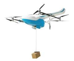
"The new Pelican leverages a hybrid VTOL airframe with no control surfaces to combine the reliability and flight stability of a multirotor platform, with the extended range of a fixed wing craft." (Photo: A2Z)
