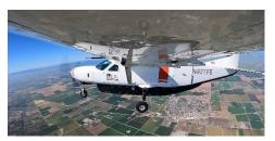
*Reliable Robotics is working to certify its remote-piloting capabilities in a modified Cessna 208 Caravan*
