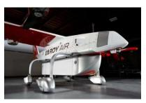
Elroy Air, the company developing the first autonomous vertical take-off and landing aerial cargo system, unveiled its preproduction Chaparral aircraft today. The Chaparral can autonomously pick up 300-500 lbs of cargo and deliver it by air up to 300 miles, a capability that pushes beyond the limited payload capabilities of delivery drones and the airport
