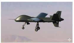
Mojave essentially takes a Gray Eagle fuselage and adds enlarged wings with high-lift devices and a Rolls Royce 450-horsepower turboprop engine. The UAS is based on the avionics and flight control systems of the MQ-9 Reaper and the MQ-1C Gray Eagle-Extended Range.
