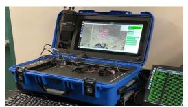
Liteye Systems, based in Denver Colorado, has partnered with Unmanned Experts Inc. to provide the hardware components to ruggedize the new AIR COMMONS™ – SWARM, drone swarm asset planning, management, and control system.
