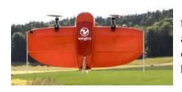
The WingtraOne is an unusual drone, both in looks and functionality. A VTOL (vertical takeoff and landing) design allows the WingtraOne to work in a wide variety of environments. Now <u>xyHt reports</u> that the Wingtra is being used to map the Alps.
