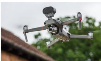
The Mavic 2 Enterprise was given its first airing at AirWorks this week. It features a compact and foldable design with an array of controls and accessories. It carries a high-resolution, 12-megapixel camera that is stabilized by a three-axis gimbal. The camera provides a 2x optical and 3x digital zoom capability.
