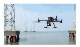
Before COVID-19 hit, San Diego Gas & Electric sent technicians up in helicopters to string power lines between towers. Now the utility has adopted DJI's Matrice 300 drones for these line-stringing operations—and no one has to evacuate. Its experience moving from manual methods to automated, drone-driven techniques is being increasingly matched across the
