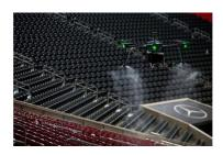
The purpose-built <u>D1 disinfecting drones</u> are being provided by Lucid Drone Technologies, and use electrostatic spraying nozzles to distribute the nontoxic disinfecting chemicals. The stadium claims it's the first professional sports stadium to use cleaning drones, and it says they reduce the time it takes to clean the stadium's seating area by 95 percent, freeing up staff to work
