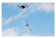
A drone releases a kevlar net to capture a simulated hostile drone during a product demonstration in Castro Valley, Calif., last year.
