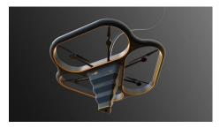
The Fly Elephant 3D printing drone would be fed printing materials through a tube at the top, to be extruded through the nozzle at the bottom
