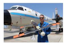
Developed for the military, Coyote is a small, expendable UAV that is air- or ground-launched into environments too dangerous for manned aircraft. The system can fly for more than an hour and up to 50 miles from its host aircraft.
