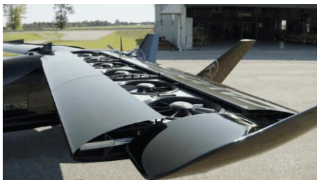
Horizon's patented fan-in-wing design for vertical lift
