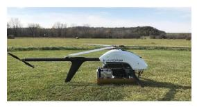
The AeroVironment Vapor 55 UAS helicopter with the high-frequency radar prototype. The radar will be used to measure surface features, particularly crevasse size and shape. The silver box is the radar, and the tan box below is the antenna.
