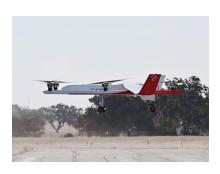
Describing it as a "flying Ford F150 truck," U.S. startup Elroy Air has begun flight-testing its Chaparral large unmanned cargo aircraft. The 1,215-lb. vertical-takeoff-and-landing aircraft made a 64-sec. first hover flight on Aug. 14 at the Camp Roberts California National Guard Base.
