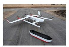
The Chaparral uses an under-fuselage cargo pod that is loaded and unloaded independently of the aircraft and then positioned on the airport ramp. The aircraft then taxis in autonomously, drops off its pod and picks up another one.
