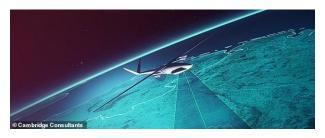
The craft weighs just 264 pounds, stretches 32 feet and runs on hydrogen that produces longer endurance but releases zero emissions.
