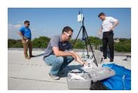
A Dedrone RF-100 drone-detection sensor on the roof of Fort Lesley J. McNair's Marshall Hall
