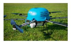
It works by the hydrogen remaining stable and solid in these structures until "coolant" is pumped through the tubes, warming them and releasing hydrogen gas to the drone's fuel cell. Hydrogen is pumped into one side of the fuel cell through a catalyst which frees electrons, creating electricity.
