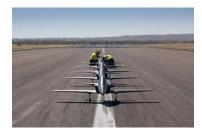
Boeing has successfully completed a series of test flights using five "high-performance surrogate jets" operating autonomously in a team. The flights, which took place over ten days, were designed to test Boeing's advanced autonomy technology including onboard command and control and data sharing capabilities. The 11-foot test aircraft reached speeds of 168 mph
