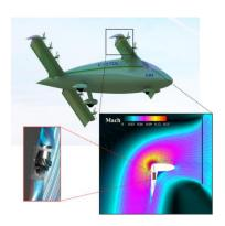
The vehicle is shown hovering with its flaps pointing downward and its propellers facing forward. The airflow from the propellers is turned vertically downward (see right inset) converting the entire thrust from the propellers to vertical lift. Unlike most of the current VTOL vehicles, the lift is generated without rotating the propellers upward. The 90 degree turn in the airflow is enabled by the coflow jet micro-compressors embedded in the flaps of all four wings.
