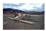
The V20, shares the same architecture and advantages of the larger V300 but is designed as a lightweight cargo courier carrying payloads of up to 20 kg. <a href="https://www.pipistrel-aircraft.com/pipistrel-begins-to-accept-orders-for-nuuva-series-of-cargo-evtol-aircraft/">https://www.pipistrel-aircraft/</a>
