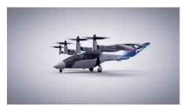
A Rolls-Royce electrical power system will be integrated into the piloted all-electric vertical take-off and landing vehicle which will carry up to four passengers for 120 miles at cruise speeds of over 200mph and is on course to certify in 2024.
