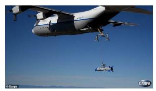
An X-61 Gremlin Air Vehicle (GAV), an unmanned reconnaissance vehicle developed by the Defense Advanced Research Projects Agency (DARPA), has been recovered while in mid-flight for the first time.
