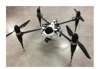
Rapid Composites has announced Bullray – a rugged, fully autonomous waterproof and manportable VTOL unmanned aircraft system (UAS) that is optionally configured for less-than-lethal applications. The aircraft can be configured as a tri-, quad-, hex- or X4-copter covering a wide spectrum of markets.
