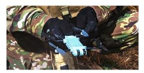
Small unmanned aircraft system (UAS) manufacturer AeroVironment on May 9 unveiled a wearable, five-ounce (140-gram) quadrotor that draws from advances in nano technology it first made with its Nano Hummingbird concept demonstrator. AeroVironment said a U.S. government customer took delivery of 20 systems in April.
