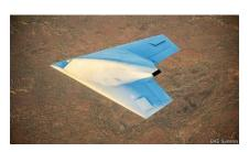
Taranis looks like something out of "Star Wars". It is about the size of a small jet fighter, but is shaped like a flying wing. It is an unmanned, stealthy combat drone. Like most military drones it can be operated, via a secure data link, by a pilot sitting in a control centre on the ground. Taranis, however, can also be let off its digital leash and allowed to think for
