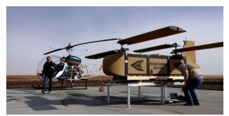
Yates Electrospace Corporation has released its Silent Arrow tactical <u>resupply drone</u> made to carry over 1,600 pounds to <u>soldiers</u> and first responders. The drone folds into itself for easy transport and a minimum set-up time required.
