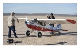
The NASA MicroCub (µCub) is a Bill Hempel 60percent-scale Super Cub, modified to support research focused on the integration of unmanned aircraft into the National Airspace System (NAS).
