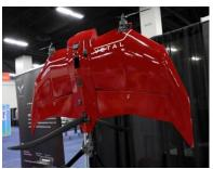
Here was a rather unique (and pricy) product. The VETAL vertical takeoff and landing drone by HiveGround is a twin-rotor drone featuring the ability to swap out payloads and a magnetic battery. It retails for \$20,000.
