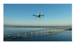
Over on Florida's Sanibel Island, which was separated from the mainland when Hurricane Ian caused a bridge to collapse, Verizon used a drone to create a popup flying cell site. The site is made up of a tethered drone outfitted with a cellular node, It was able to provide coverage for a 5–7-mile radius. Since it's tethered, it can fly for up to 1,000 hours.
