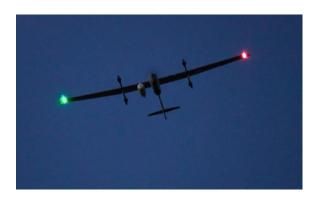
A production Stalker VXE was configured with an external, wing-mounted fuel tank for the 39 hours, 17 minutes, and 7 seconds flight — a record in the Group 2 unmanned aerial system category (11 to 55 pounds).
