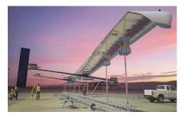
Ordnance Survey and a team of aeronautic engineers are developing an innovative solar powered, High Altitude Pseudo Satellite to change how the planet is mapped.
