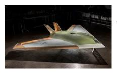
The Magma drone is controlled by blasts of air taken from its jet engine and blown over its wings
