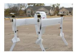
The model flown has a fixed pod, but modularity is one of the major aims of the APT program, with sketches showing much larger multirotor versions and even gimballed storage pods, so that the orientation of the cargo remains the same from vertical takeoff through midair transition and back again to landing. And the capacity imagined is extensive, with cargoes of 500-1,000 lb.
