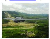
**Lockheed Martin's** Fury, an advanced tactical Group 3 unmanned aerial system, is regularly flying long-range endurance test missions as the company prepares it for low-rate production. Since May 2016, Fury has flown 200 hours in flight tests and demonstrated 12-hour endurance with 100 pounds of payloads including electro-optical/infrared surveillance systems, voice communications relays, SATCOM links, and
