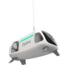
Zipline's nearly-silent <u>Platform 2</u> Zip drones fly over 300 feet above ground, hovering safely above their destination, where its autonomous delivery droid drops off payloads using a tether. The Platform 2 is usable for delivery within a 10- mile service radius, as well as as a network in which Zips can travel up to 24 miles each way from dock to dock, extending a business' reach.
