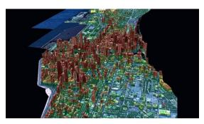
LiDAR, or Light Detection and Ranging, is a way to measure ground elevation with light with millimeter accuracy. The process works by shooting a light beam down at the surface and then measuring the light that returns after being reflected by the ground. The sensor can also detect changes made to the light if it passes through the foliage, like trees
